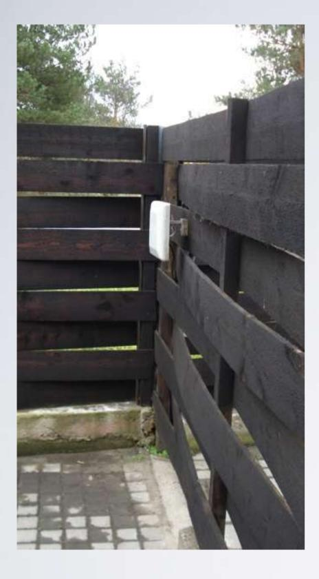
FMW 3/1 2.45 GHz FMW 3/1 is an economy model of Perimeter Detectors. This detector offers a maximum detection range of 100 meters. the detection zone is up-to 1.8 meters in height and 5 meters in width.
